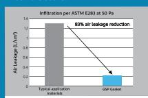
Third-party testing shows GREAT STUFF PRO  $^{\rm TM}$  Gasket achieves a 83% air leakage reduction over wet-applied caulk.
